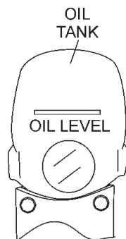
Figure 7. Oil Tank (Front View)
