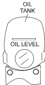
Figure 9. Oil Tank (Front View)
