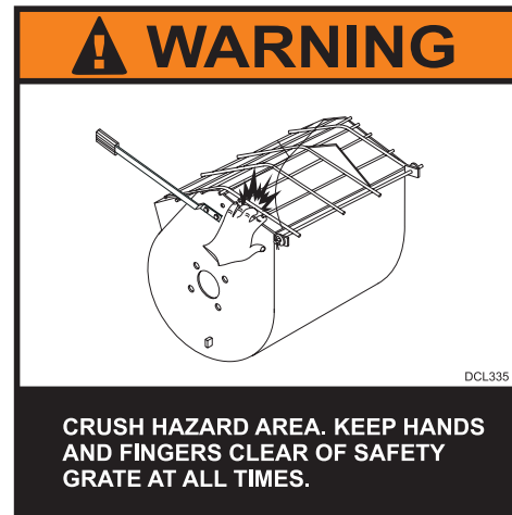
Figure 37. Safety Grate (Crush Hazard)
