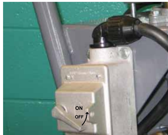
Figure 8. Electric Motor ON/OFF Switch
