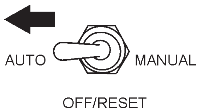
Figure 53. MPEC Control Switch (AUTO)
