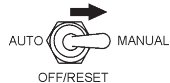
Figure 42. MPEC Control Switch (Manual Position)
