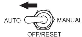
Figure 55. MPEC Control Switch (AUTO)
