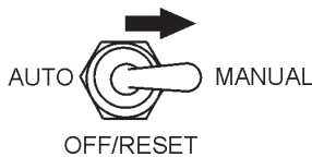
Figure 41. MPEC Control Switch (Manual Position)
