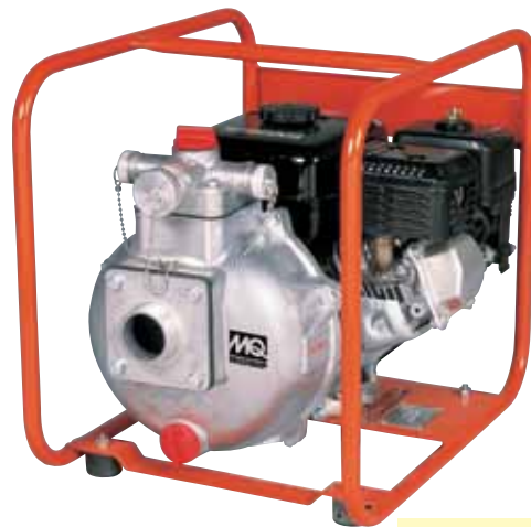
QP205SH 2" Suction - 100 psi. 106 GPM - 230' HEAD
