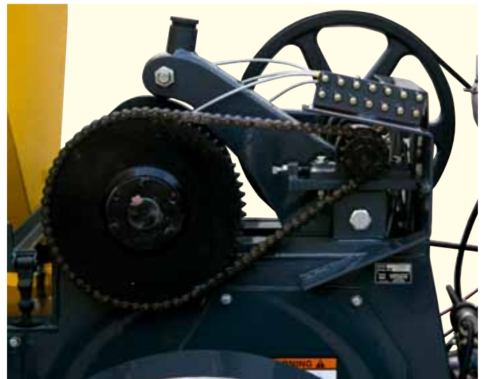
Central lubrication system for quick and easy maintenance.
