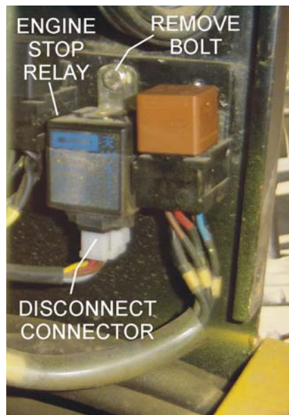
Figure 5. Engine Stop Relay Removal/Installation
