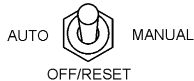
Figure 56. MPEC Control Switch (Off/Reset)
