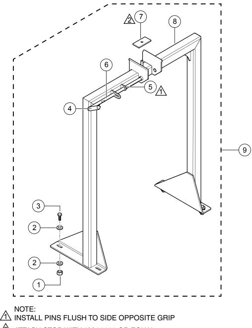
ATTACH STOP WITH 3M 08008 OR EQUAL WEATHERSTRIP ADHESIVE.
