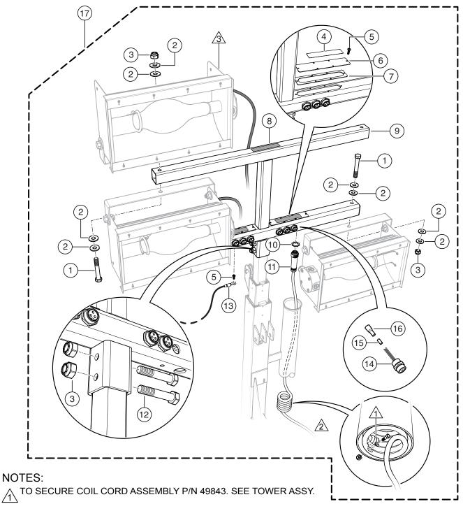
CONNECT THIS END OF COIL CORD ASSEMBLY TO BALLAST BOX. SEE COIL CORD ASSY.
