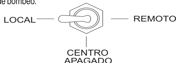
Figura 26. Interruptor de control de bombeo (LOCAL)
