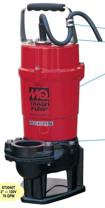
Heavily debris-laden water calls for rugged pumps. Submersible trash pumps are equipped with a 2" discharge port and easily handle solids up to one inch in diameter. A vortex action discharges solids away from the cast iron multi-vane impeller to prevent clogging.
