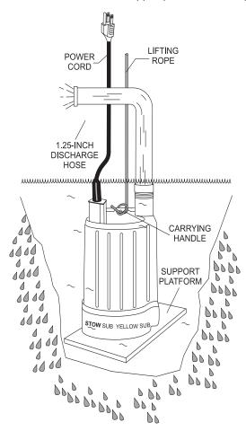
Figure 2. Submersible Pump Upright Position (Correct)
