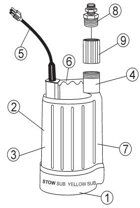
Figure 1. Submersible Pump Components
