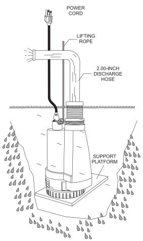
Figure 2. Submersible Pump Upright Position (Correct)
