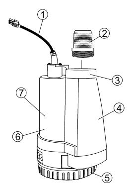
Figure 1. Submersible Pump Components
