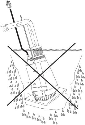
Figure 3. Submersible Pump Upright Position (Incorrect)
