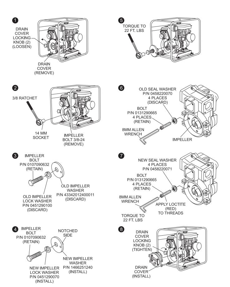
Figure 1. Impeller/Seal Washer Installation
