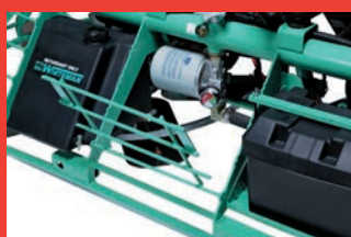
Hinged panels make servicing easy by allowing quick access to filters and trowel blades
