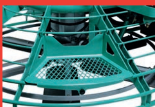
Removable steps provide quick access to trowel blades
