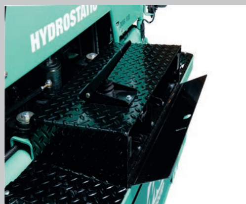
Raised operator's platform includes lockable storage compartment
