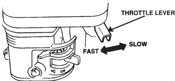
**Figure 30. Throttle Lever**
