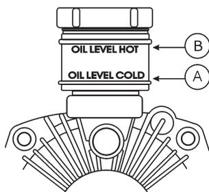
**Figure 9. Transmission Reservoir**
