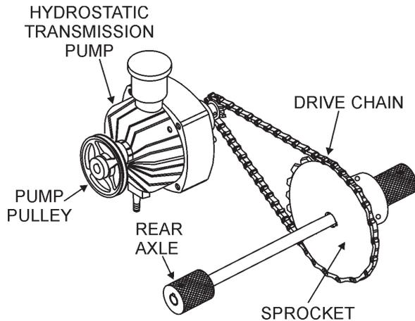
**Figure 8. Hydrostatic Transmission**
