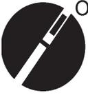
**OFF** **ALWAYS** place the **ON/OFF** switch in the **OFF** position, remove key and/or disconnect the spark plug lead before servicing the engine or equipment. Ground the lead to prevent sparks that could ignite a fire.
