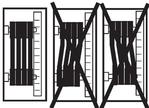
Figure 49. V-Belt Alignment
