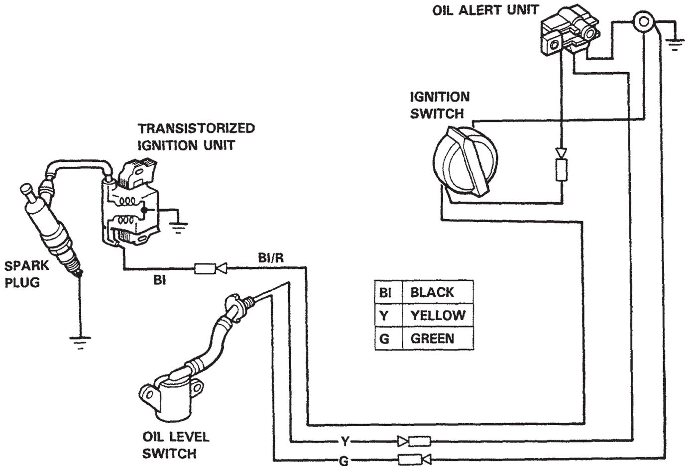
Figure 52. 13HP Honda Engine Wiring Diagram
