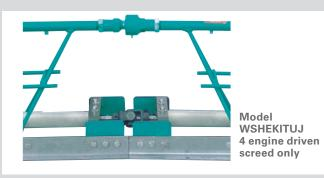
**Universal Joint Kit** – Designed exclusively for engine-driven screeds, this kit contains a ball-joint coupler for the screed top pipe and a universal joint for the eccentric shaft. Installed between two screed sections it allows for crowns or inverts up to ¼-inch per foot without extending the overall length of the screed.
