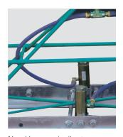
Naval bronze air vibrators are rust resistant and deliver high frequency vibration.
