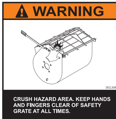
Figure 38. Safety Grate (Crush Hazard)
