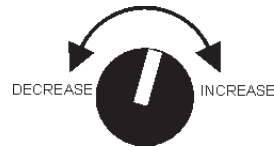
FIGURE 35. Voltage Regulator Knob located on the control panel
