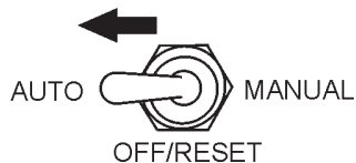
Figure 55. MPEC Control Switch (AUTO)
