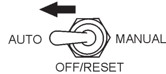
Figure 41. MPEC Control Switch (AUTO)
