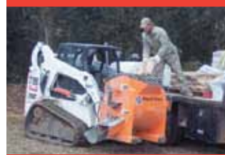
Very easy to load. Move the mixer to where the materials are.
