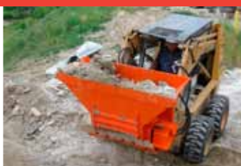
Level Hog Crusher and start recycle process.
