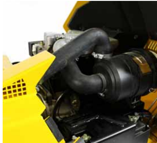
New air intake design located at the highest point for optimal performance.
