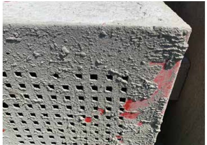
Built-up concrete or mortar makes equipment look old and worn-out.
