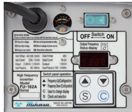
FU162A Control Panel
