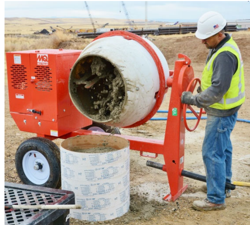
Polyethylene drum 9CF Concrete mixer
