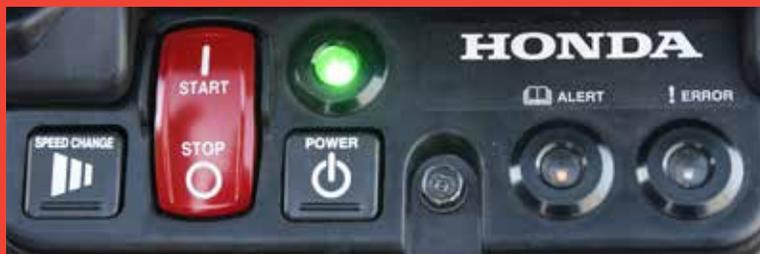
The rammer control panel offers simple startup and speed controls along with LED warning indicators.
