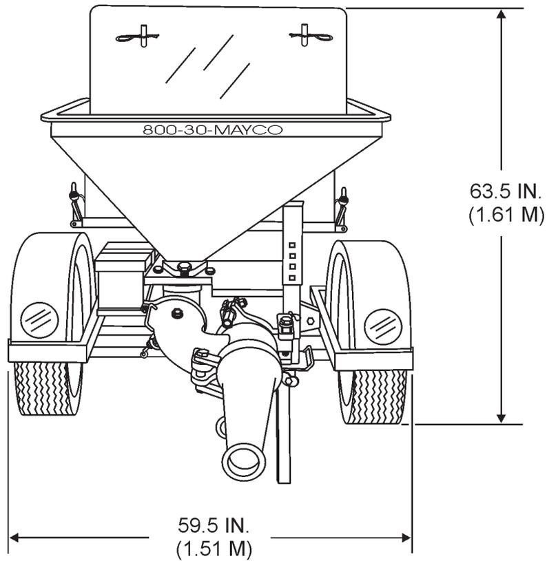
Figure 1. C-30HDG Concrete Pump Dimensions
