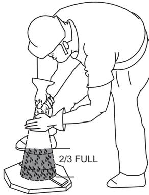
Figure 41-B. Slump Test (2/3 Full)
