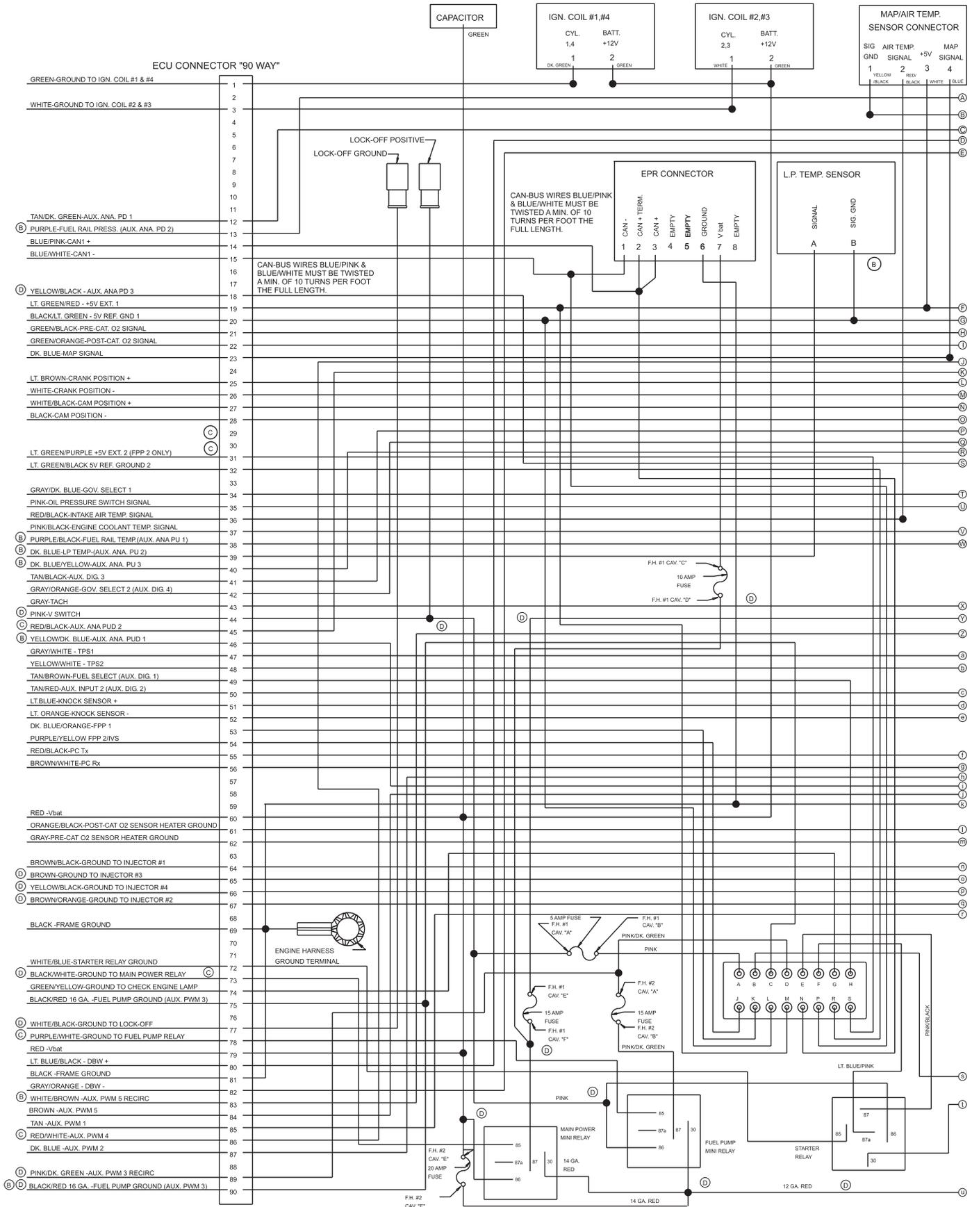
Figure 38. Zenith Fuel Injection System Wiring Diagram
