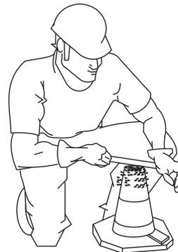
Figure 41-D. Slump Test (Removing Excess Concrete)
