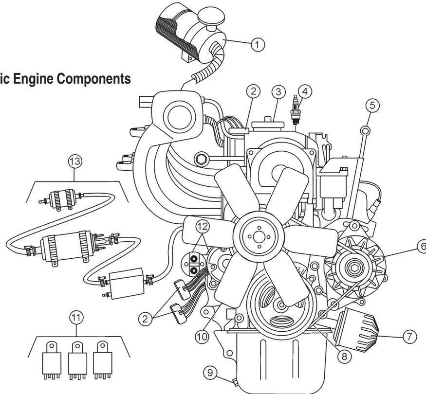
Figure 9 illustrates the location of the basic components for the Zenith 416, 1.6 liter gasoline engine. The function of each component is described below:
