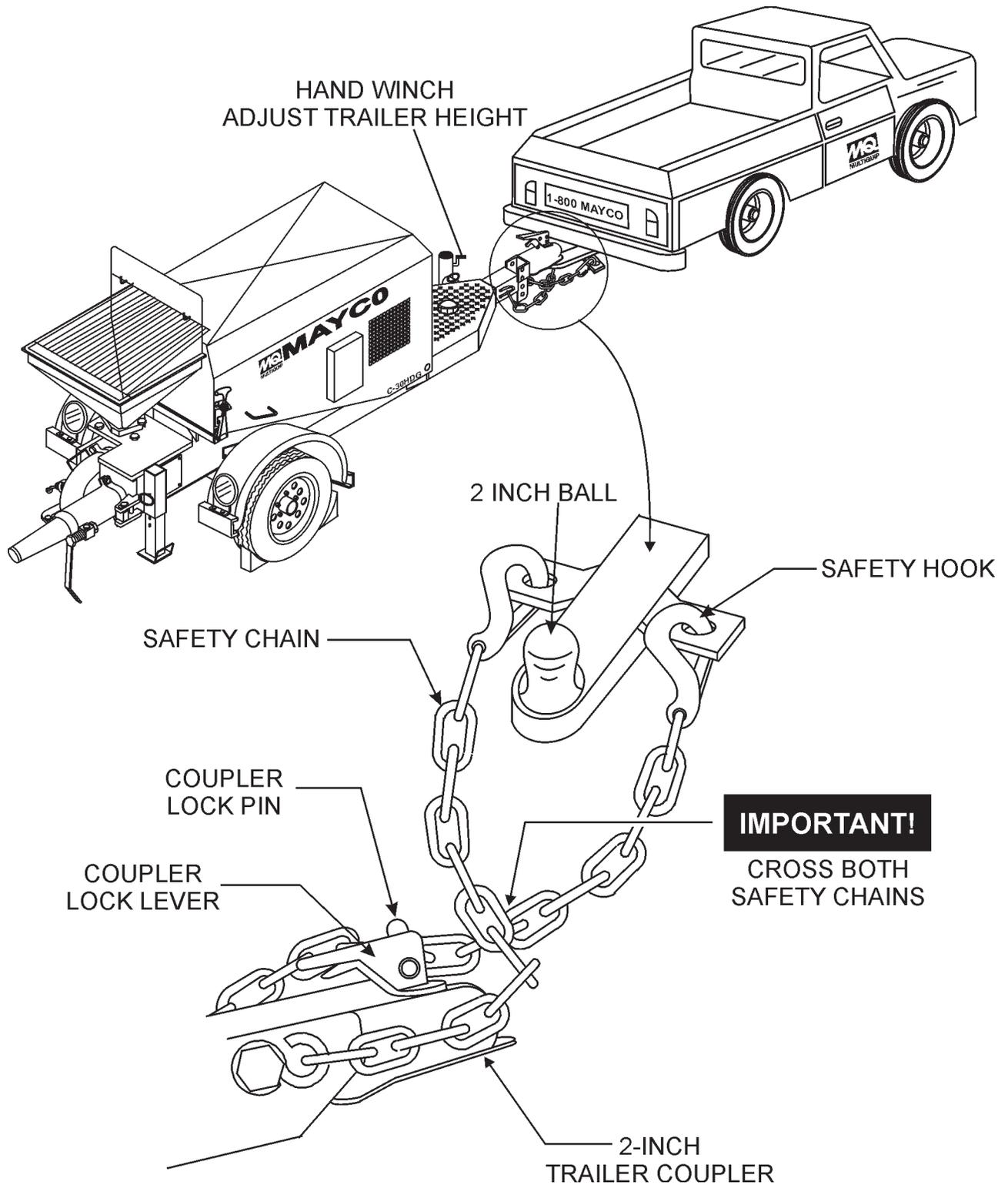
Figure 2. Towing Applications
