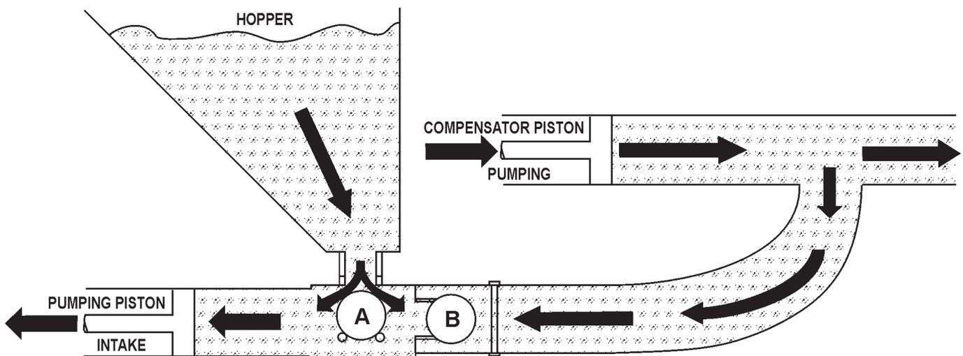
Figure 10. Pumping Cylinder
