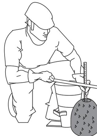
Figure 41-F. Slump Test (Measurement)
