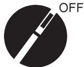
**ALWAYS** place the **Engine ON/OFF** switch in the **OFF** position and remove the ignition key when the pump is not in use.
