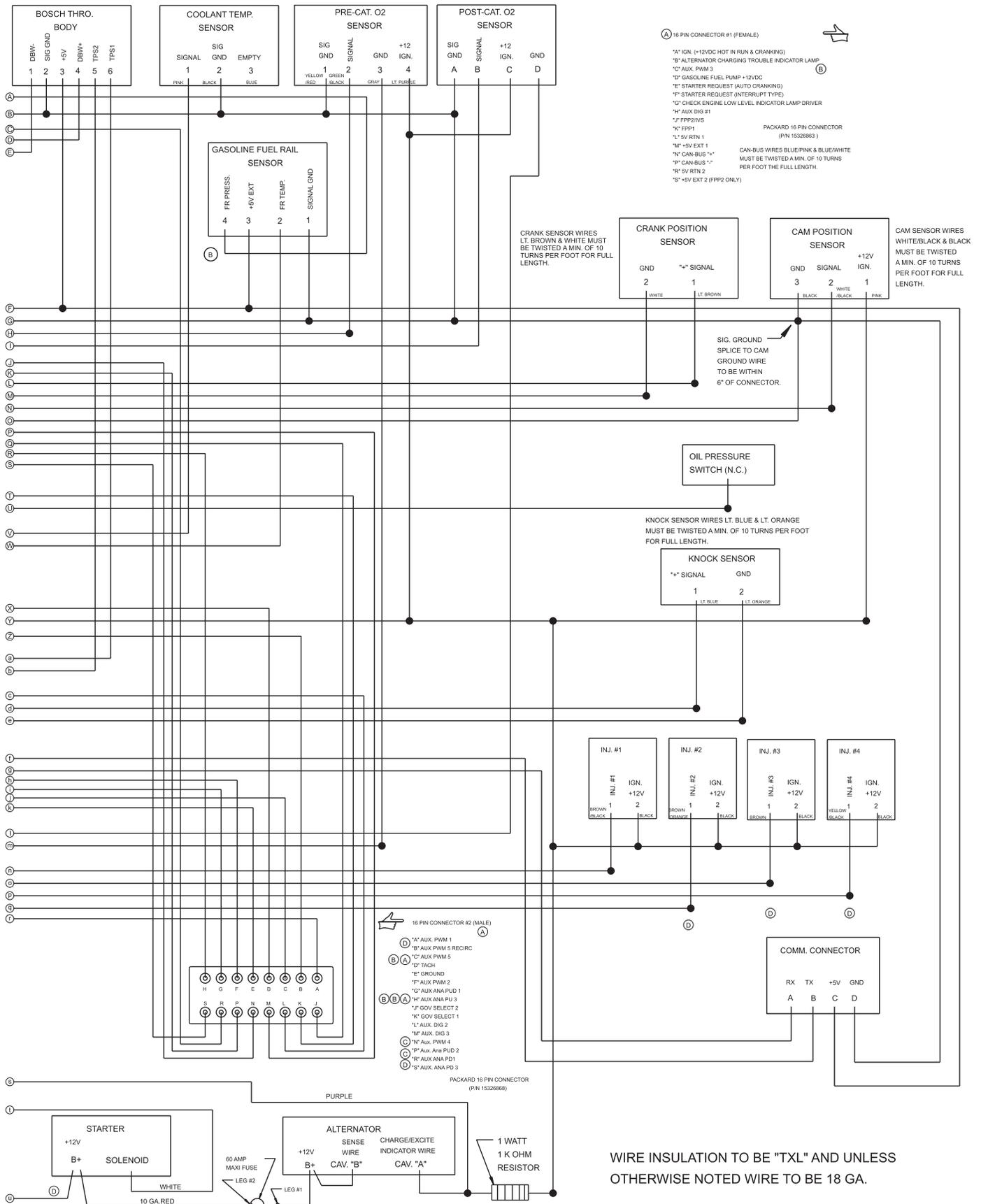
Figure 38. Zenith Fuel Injection System Wiring Diagram (Cont.)
