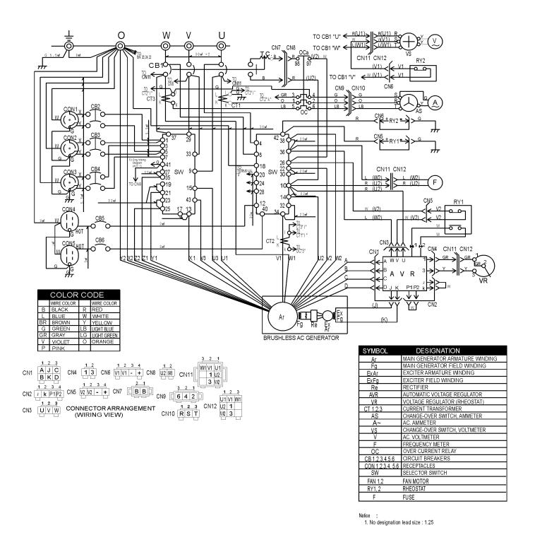
Figure 65. Generator Wiring Diagram
