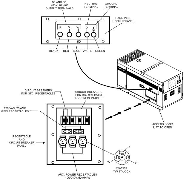
**Figure 6. Output Terminal Panel**
