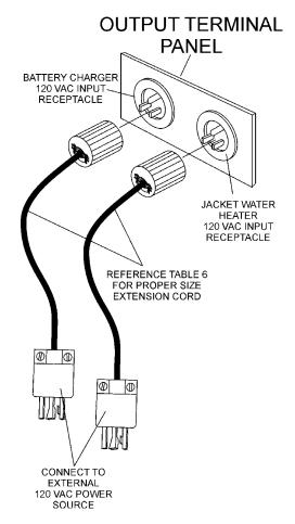
Figure 60. Battery Charger & Jacket Water Heater Power Connections
