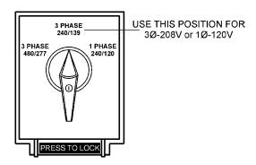
Figure 22. Voltage Selector Switch 3Ø-240/139V Position
