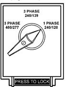
Figure 38. Voltage Selector Switch STARTING (MANUAL)
