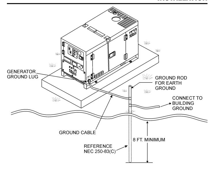
Figure 2. Typical Generator Grounding Application
