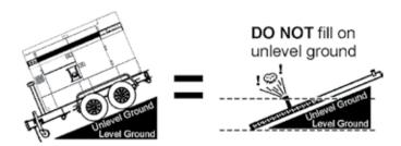
Figure 30. Only Fill on Level Ground
