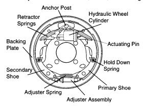
Figure 61. Hydraulic Brake Components Actuator
