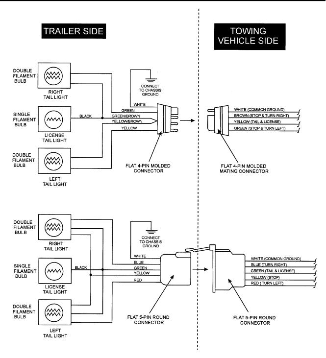
Figure 64. Trailer/Towing Vehicle Wiring Diagram
