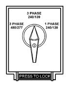
Figure 13. Voltage Selector Switch
