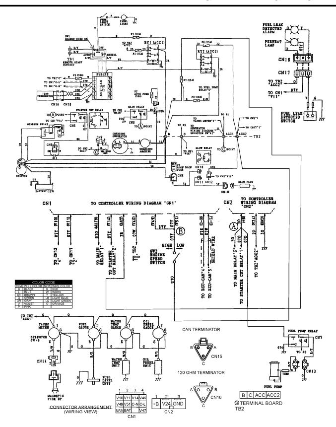
Figure 66. Engine Wiring Diagram
