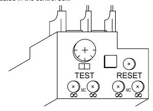
Figure 12. Over Current Relay
