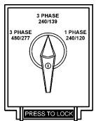
Figure 14. Voltage Selector Switch 240/139V 3Ø Position
