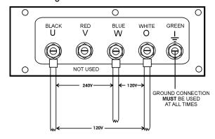
Figure 27. UVWO Terminal Lugs 1Ø-240/120V Connections
