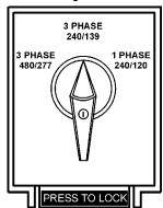
Figure 19. Voltage Selector Switch 3Ø-240/139V Position
