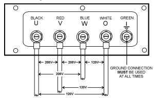
Figure 23. UVWO Terminal Lugs 3Ø-208/1Ø-120V Connections
