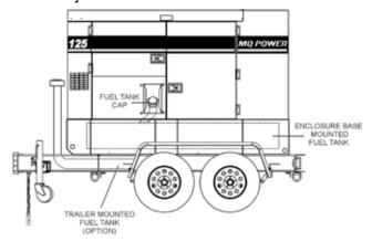
Figure 29. Internal Fuel Tank System
