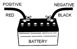
Figure 35. Battery Connections
