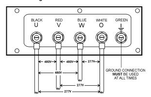
Figure 25. UVWO Terminal Lugs 3Ø-480/277V Connections
