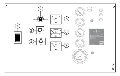
**Figure 4. Generator Control Panel**
