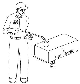
Figure 58. Fuel Tank Cleaning
