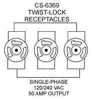
Figure 8. 120/240V Twist-Lock Auxiliary Receptacles
