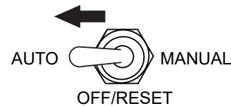
Figure 16. Auto Start/Stop Switch (Auto Position)
