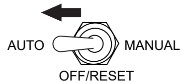
Figure 57. Auto Start/Stop Switch (Auto Position)
