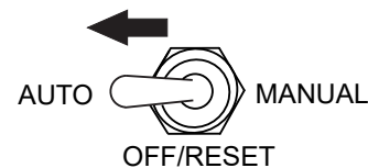
Figure 19. Auto Start/Stop Switch (Auto Position)
