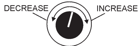
Figure 17. Voltage Regulator Control Knob
