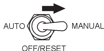
Figure 85. Auto-Off/Reset Manual Switch (Manual Position)
