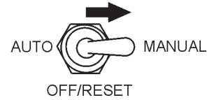
Figure 46. Auto-Off/Reset Manual Switch (Manual Position)
