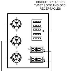
CS-6369 TWIST-LOCK RECEPTACLES (3) 240/139V, 50 AMPS GFCI RECEPTACLES (2) 120 VAC, 20 AMP
