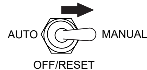
Figure 43. Auto Start/Stop Switch (Manual Position)
