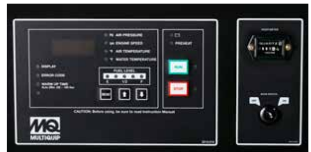
LED Digital Controller monitors compressor and engine temperature, air pressure, and fuel level. It also includes an hourmeter and provides complete engine diagnostic tools.
