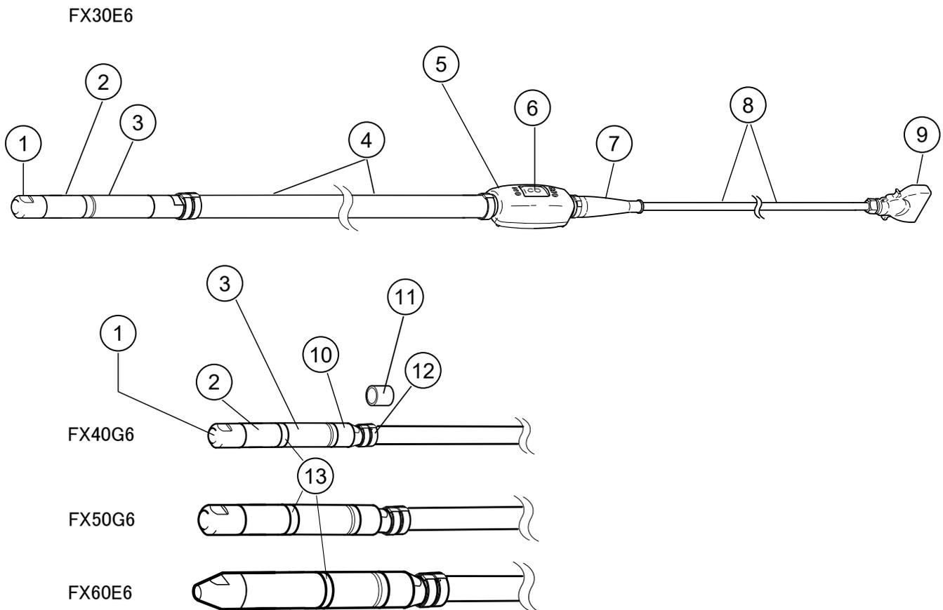
**Figure 2. Vibrator Components**
