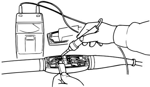
**Figure 4. Switch Insulation Resistance Check**
