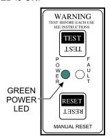
Figure 40. GFCI Module (Green LED ON)
