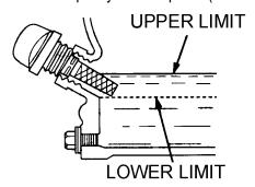
Figure 11. Engine Oil Dipstick(Oil Level)
