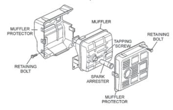
Figure 36. Spark Arrester Removal
