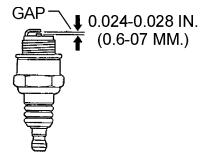
Figure 32. Spark Plug Gap
