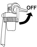
Figure 29. Engine Fuel Valve Lever (OFF)
