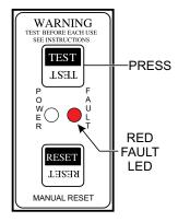
Figure 41. GFCI Module (Red/Fault LED ON)
