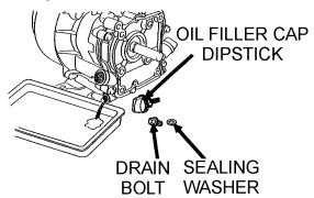
Figure 33. Draining Engine Oil
