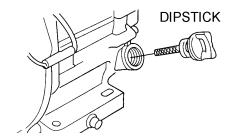
Figure 10. Engine Oil Dipstick Removal
