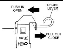
Figure 15. Choke Lever
