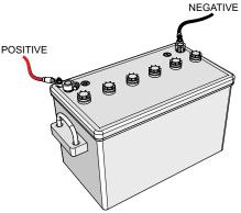
Figure 38. Battery Connections
