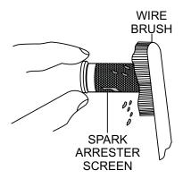
Figure 37. Cleaning The Spark Arrester
