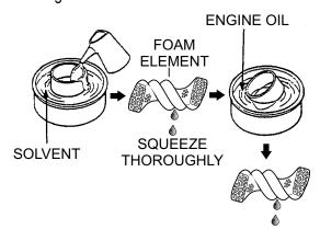
Figure 35. Cleaning Foam Element
