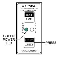
Figure 44. GFCI Module (Green LED ON Reset)
