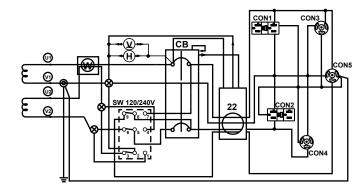
Figure 7. 240/120V Full Power Switch Simplified Diagram (Down Position)
