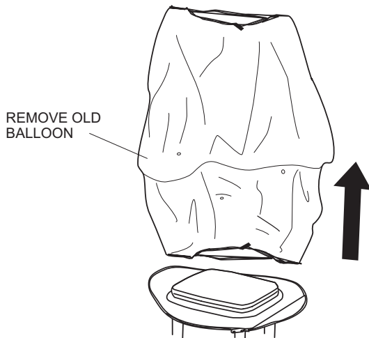
Figure 39. Removing Old Balloon
