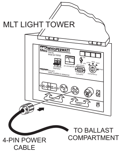
Figure 31. MLT Ballast 4-pin Power Cable
