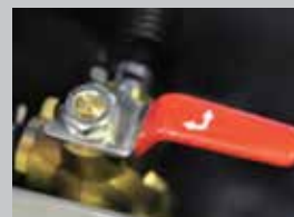
Three-way valve available to switch to external fuel tank
