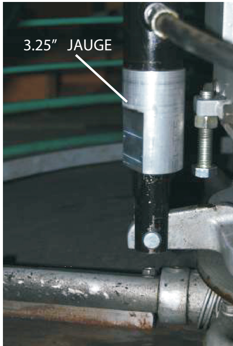
Figure 42. Installation de la jauge
