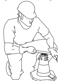
Figure Q. Slump Test (Removing Excess Concrete)
