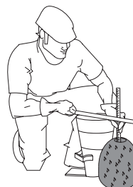
Figure S. Slump Test (Measurement)
