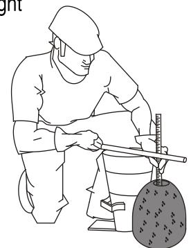
Figure 68-F. Slump Test (Measurement)
