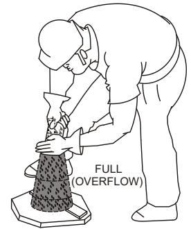
Figure 68-C. Slump Test (Full-Overflow)
