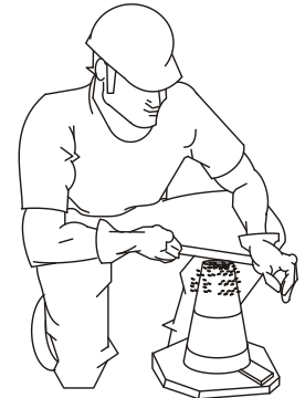
Figure 68-D. Slump Test (Removing Excess Concrete)
