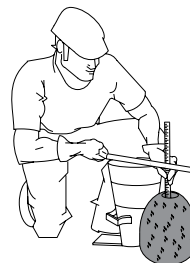
Figure S. Slump Test (Measurement)
