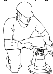
Figure Q. Slump Test (Removing Excess Concrete)
