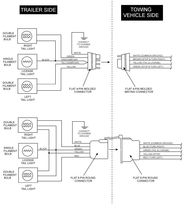
Figure 10. Typical Trailer Wiring Diagram
