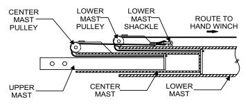
Figure 21 Mast Extension Cable System
