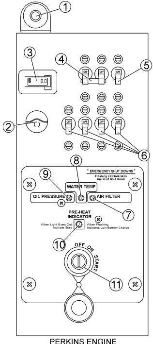
PERKINS ENGINE CONTROL PANEL Figure 5. Control Panel Components and Indicators
