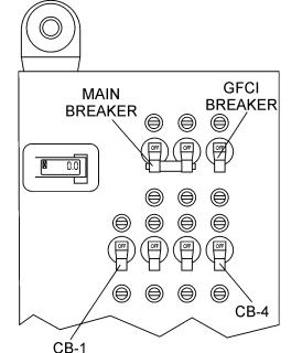
Figure 17. Control Panel Circuit Breakers
