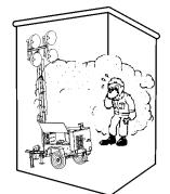
enclosed or narrow area where free flow of the air is restricted. If the air flow is restricted it will cause serious damage to the generator engine and may cause injury to people. Remember the engine of the light tower/generator gives off **DEADLY** carbon monoxide gas.
