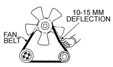
Figure 14. Fan Belt Tension
