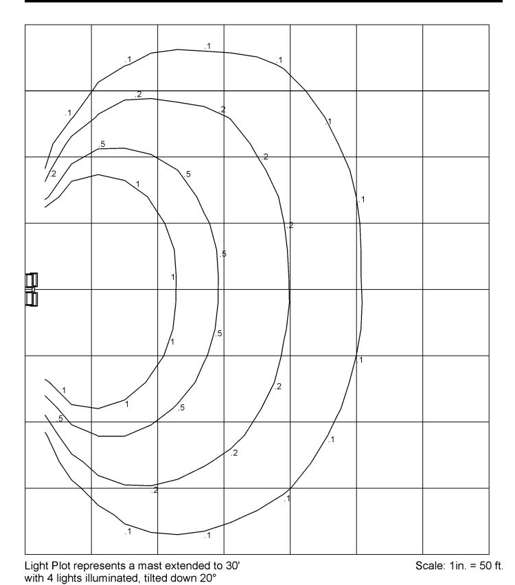
Figure 6. Floodlight Footcandle Plot (Area Coverage)
