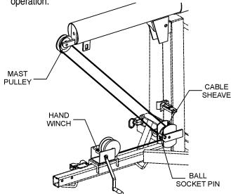
Figure 20. Mast Raise/Lower Cable System
