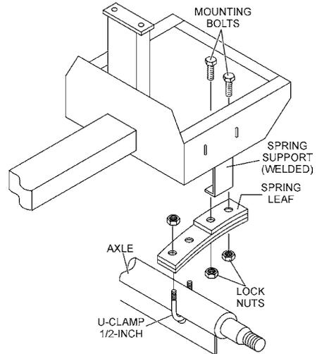
Figure 37. Suspension Components
