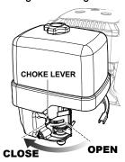
Figure 24. Choke Lever
