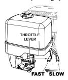
Figure 25. Throttle Lever
